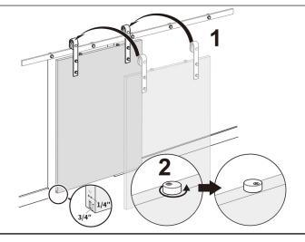
STEP 07: Stoppers can be placed inside the end mounting track bolts to shorten the sliding movement
