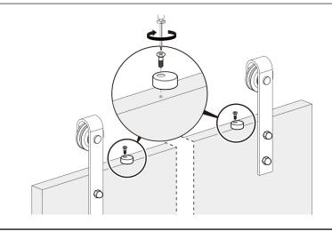
STEP 06: Install the floor-mount guide
